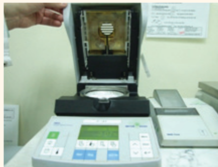
b. Sample pan is placed in the heating chamber and integrated balance.
