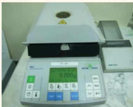
c. The heating chamber is closed and start button is pressed.
