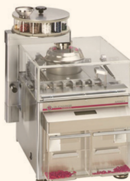
Fig 3.7 Automatic measuring equipment- weight, thickness and hardness
