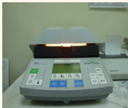
d. Drying process in progress and the balance periodically weighs the sample.
