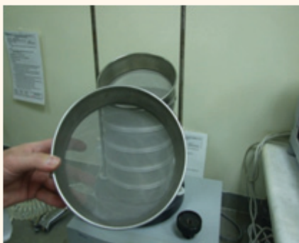
a. Stacking the sieves on top of one another.
