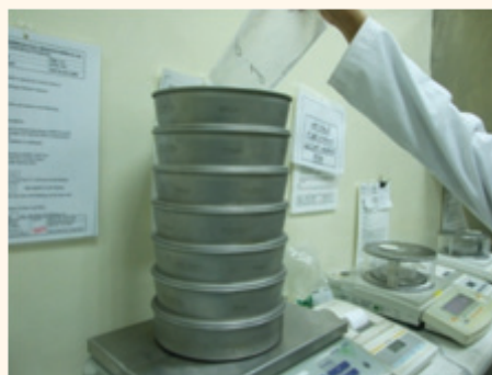
a. Placing the test powder on the top sieve.
