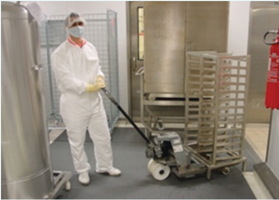
Fig 2.1 Contamination controlled handling
